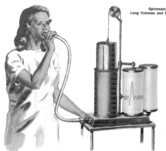
Figura 2. Espirómetro de Campana (Del manual CIBA Collection of Medical Illustrations Vol 7)
